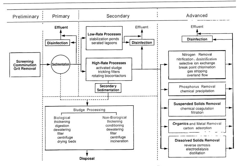
Figure 1 — Generalized Flow Sheet for Wastewater Treatment Source: Asano, T., R. G. Smith, and G. Tschobanoglous, 1984
